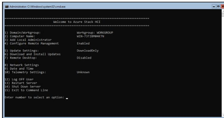
Figure 2 - SCONFIG in Azure Stack HCI
